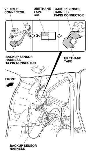
44. Using scissors, cut one urethane tape as shown. Attach the cut piece of urethane tape to the backup sensor harness 13-pin connector.
