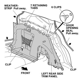
17. Release the cable, then remove the left rear seat release lever (two clips and five retaining tabs). Remove the left rear side trim panel.
