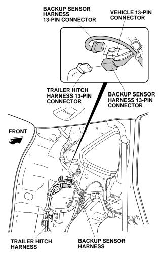
47. Plug the trailer hitch harness 13-pin connector into the backup sensor harness 13-pin connector. Go to step 50.
