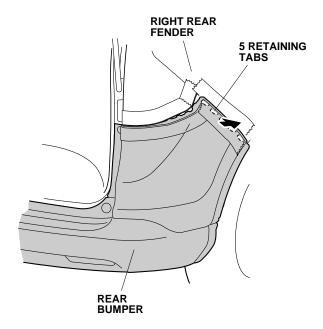
Release four retaining tabs on each side.
