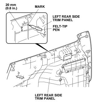
56. Using a utility knife, cut out the ribs on the left rear side trim panel. Remove any burrs.
