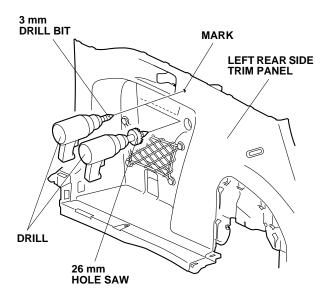
59. Install the switch into the 26 mm hole in the left rear side trim panel. Make sure the switch is installed right side up.
