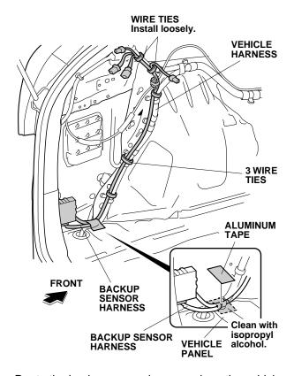
Route the backup sensor harness along the vehicle harness. Secure it to the vehicle harness with five loosely-installed wire ties as shown. Go to step 42.
