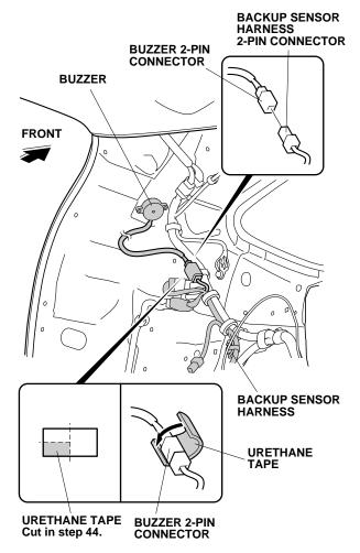
53. Attach the other piece of urethane tape (cut in step 44) around the buzzer 2-pin connector.
