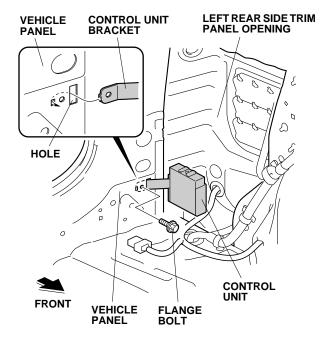
37. Plug the backup sensor harness 14-pin connector into the control unit.
