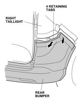
With the help of an assistant, remove the rear bumper. Place the rear bumper on a blanket.
